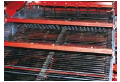
1650mm wide main web and second web for improved separation.
