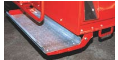
The operator's platform can easily be folded up to reduce transport width.
