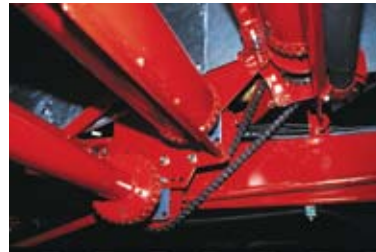
The 3 roller positive main web drive system facilitates easy changing of webs to suit different crop and field conditions.
