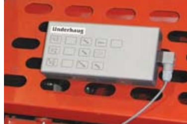
Control panel for picking table.
