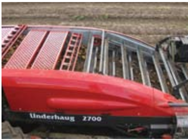
Flight conveyor on main web (option). Extra cleaning. Stops the crop from rolling back.
