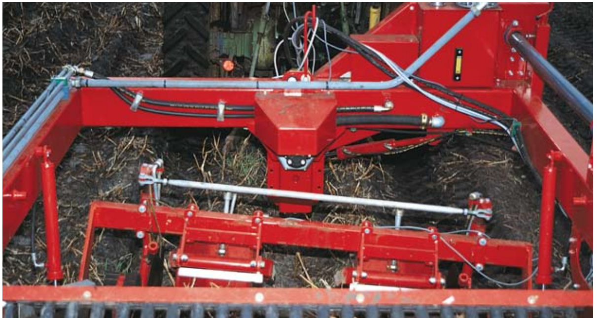
Unique floating lifting unit follows the ground contours.
